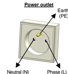
3. To test the tripping of the 30mA ground fault switch, connect the tester to the wall outlet and check that the wiring is correct. Press the ground fault generator button. If the ground fault switch is operational the power will be cut off (< 3 s). If there is no earth connection the ground fault switch will not cut off the power.
