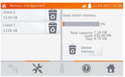
This option allows you to read the % of the used memory and to clear it: after clicking Delete memory all clients are deleted with their objects and measurement results. By pressing button located next to each customer, you can also delete individual customers.
