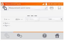
The measurement is performed as in the case of testing the inductive objects If based on the difference between the instantaneous and average resistance during the result stabilization, the meter determines that the object is resistive, it will complete the measurement faster.
