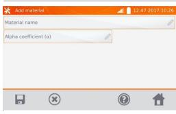
Enter and save the material and  $\alpha$  coefficient, using the same method as described in section 2.2.4.
