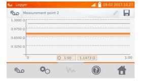
Use who button to display the graph of resistance over time - both during the logging process and after its completion.
