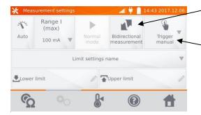
Switching Unidirectional/Bidirectional measurement.
