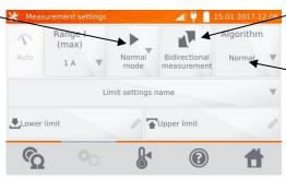
Switching Unidirectional/Bidirectional measurement.
