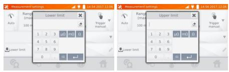
Click \( \bigset^\* \), to enter the temperature settings. After checking "Temperature compensation" box, the meter uses the specified temperatures and temperature coefficient of resistance to calculate the resistance at the reference temperature.
