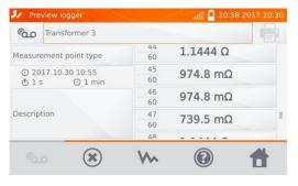
When using the logger, clicking the field with results will cause the meter to display the individual samples. You may scroll them using , buttons. Use button to display the graph.
