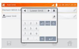
Enter the lower limit. Use button to go to the upper limit setting. You can also set only one of the limits.
