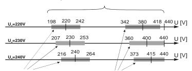
The voltage range U <sub>L-N</sub>, for which the short-circuit current is calculated
