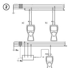
Connect test leads according to the drawing
