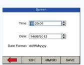
Use the rotary encoder to change the Time/Date and press function key F4 to Save
