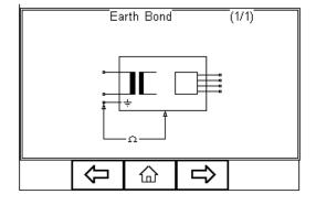
If an earth bond lead other than that supplied with the Rigel 62353 Plus is to be used then any resistance associated with this lead can be zeroed out by connecting the supplied earth bond lead to the EUT earth socket on the Rigel 62353 Plus and
