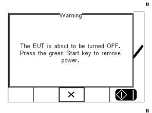
The next step is to reverse the power supply. The Rigel 62353 Plus will automatically reverse the power and start the test sequence again. In the semi automatic mode, the user can determine when the measurements start. In full automatic mode, the power reversal is instant and measurements will start directly after mains reversal.
