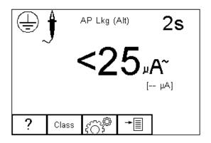
Press Duration, Equipment Class, Applied Part module and RMS Pass/Fail limit for BF and CF Applied Parts. Use the up, down. left and right keys to highlight and set. Press (F4) when complete. Pressing the button (F3) will exit Settings mode without saving changes.
