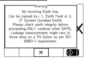
In addition, the Rigel 62353 Plus is able to check for a valid test setup for measurements done using the direct method. In case a secondary earth path is detected, the Rigel 62353 Plus will warn the user. It is *not possible to continue* as testing under such conditions will always result in a "zero" reading due to the low Ohm resistance of the secondary earth path in comparison to the 1000 Ohm resistance of the body model used in the Rigel 62353 Plus.
