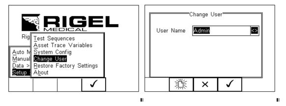
Select a different user using the drop down menu or create a new user name by pressing the button (F1) .
