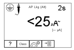
Press to set the Test Duration, Insulation test voltage (500 / 250VDC) and Pass/Fail limit. Use the up, down, left and right keys to highlight and set. Press button (F4) when complete. Pressing button (F3) will exit Settings mode without saving changes.
