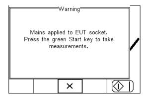
This example uses the Semi Automatic Mode and the user has the opportunity to determine the moment at which the leakage measurements start. In fully automatic mode, the Rigel 62353 Plus will start the measurements immediately after the EUT has been switched on.
