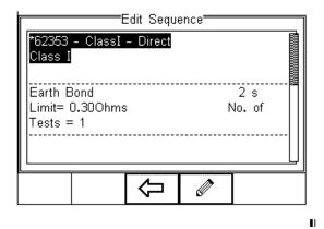
To change the Name and or Class of the Test Sequence, press the and enter the Name and or Class required.
