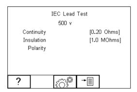
Press (C) button (F3) to set the Pass/Fail limits for Continuity, Insulation and Test Voltage. Use the up, down, left and right keys to highlight and set. The pass/fail limit for the continuity stage can be calculated using the Calc button (F2). Enter the type and length of cable and a new limit will be calculated. This can be overridden by selecting
