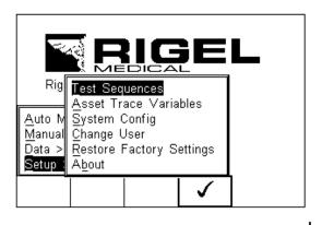
The following screen displays the list of default and customised tests available. Copied Test Sequences will appear in the list with an \*pre-fix.
