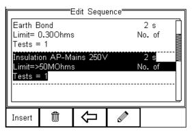
Further electrical safety tests can be inserted or deleted by following the steps described herein.
