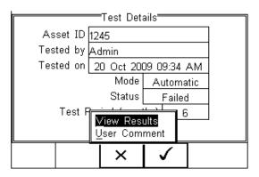
**View Results** will display the results of the test (see section 3.6)
