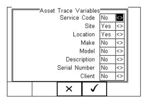
The default settings on the Rigel 62353 Plus include the Site and Location variables. Both are activated. The drop down box is set to [Yes].
