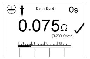
Caution, never connect the Earth Bond Probe to voltages in excess of 30V since this can cause damage to the equipment.
