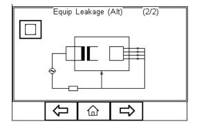
The test is performed using current limited (3.5mA) mains potential sinusoidal 50Hz signal. (60Hz where this is the mains frequency)
