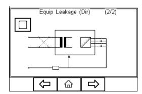
All Applied Parts and earthed (eg enclosure Class I) and non-earthed accessible conductive parts or non-conductive accessible parts (enclosure Class II) are grouped together and connected to earth via the  $1k\Omega$  Measuring Device (Body Model).
