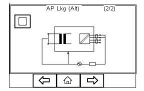
The test is performed using a current limited (3.5mA) mains potential sinusoidal 50Hz signal. (60Hz where this is the mains frequency)
