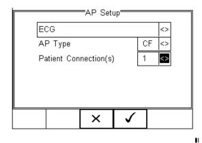
When the configuration has been completed, press the button (F4). Pressing the button (F3) would return to the previous screen and lose the settings.
