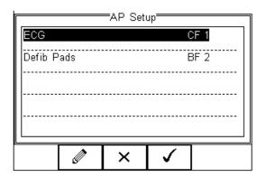
When the configuration has been completed, press the button (F4). Pressing the button (F3) would return to the previous screen and lose the settings.
