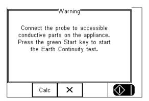
Attention! Ensure the earth bond test lead is connected to the black socket when testing between probe and EUT earth.
