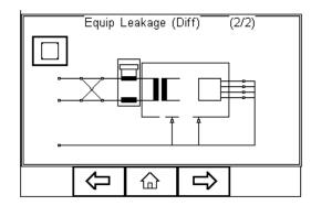
Measurements are done in both polarities of the incoming mains with the protective earth to the EUT interrupted.
