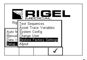
All the settings provided within the Setup menu will default to Factory Settings including; All Asset Trace Variables, Test Sequences, User Admin and System Config.
