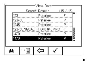
Use the up and down arrow keys to scroll through the database. When the desired record is highlighted, press the data.
