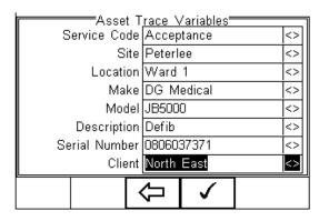
8. Use the Up & Down Keys to navigate the menu and the Left & Right Keys to open the drop down boxes [<>]. Select the required input and confirm with the
