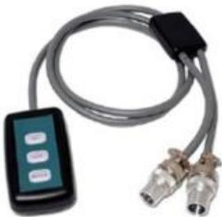
**CQM Cable Differences** – Two CQM cables are provided in the standard accessory kit. The only difference between them is that one cable has a small pin and the other does not. The cable with the pin is used to enable the REM circuitry on the DUT. The cable without the pin is used to bypass the REM circuit and allow for shorting of the REM leads. Note that some generators do not allow for the REM circuit to be disabled. For these generators it does not matter which cable is used.
