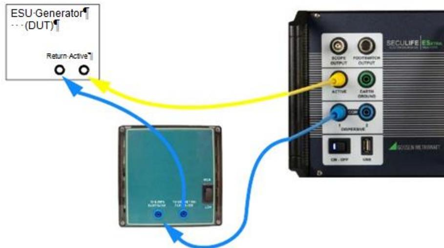
If the output terminals of the DUT are not compatible with the standard ES PRIME safety test leads, the alligator clips supplied with the ES PRIME accessory kit can be used to connect directly to the electrosurgical instrument as shown in the connection diagram below.
