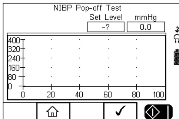
To initiate the test, press ✓ (F4). The UNI-SIM will inflate the system until the protection valve is activated;
