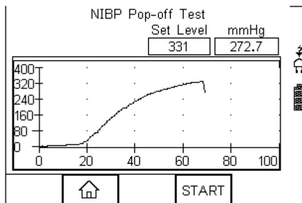
Following the Overpressure valve test, the UNI-SIM is ready to make all simulations as per the test routine;
