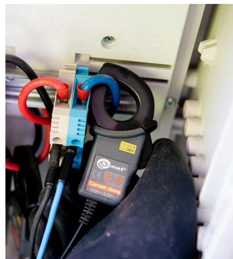
The gap (formed by the faces of the core) should be kept perfectly clean.
