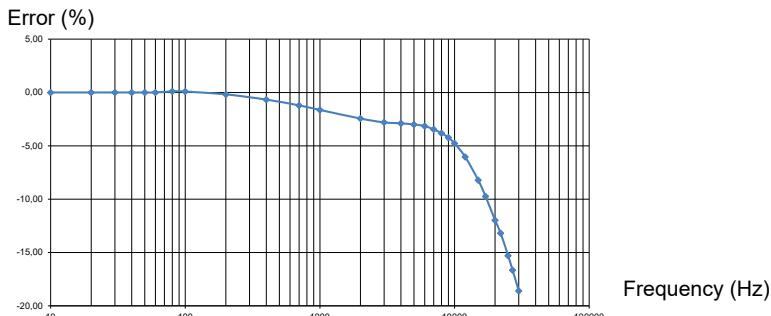
Typical phase versus frequency error curve at 60 A
