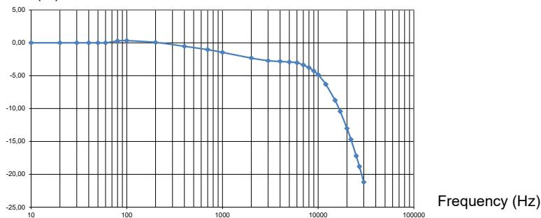
Typical phase error versus frequency curve at 30 A
