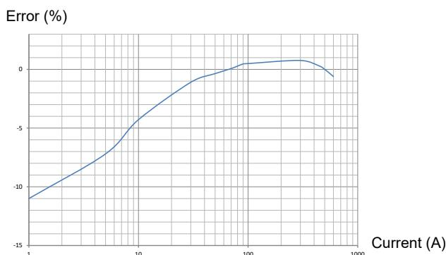
Typical phase error curve at 60 Hz
