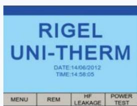
From the start screen use the rotary encoder or function key F1 to select Menu
