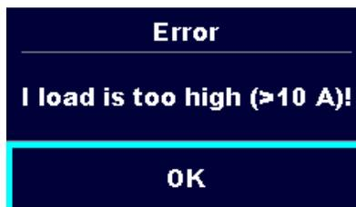
The average load current higher than 10 A over the last 5 min test interval is detected. Measurement is stopped. Recovery period for cooling is required before proceeding with tests! Press OK to continue.
