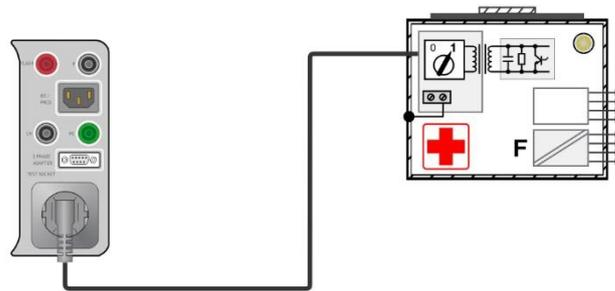
Insulation resistance – LN-PE
