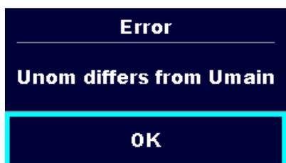
The set  $U_{nom}$  differs too much from the measured mains voltage. Parameter or mains voltage must be changed.
