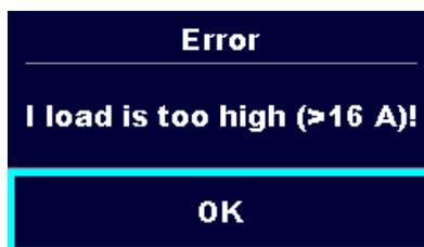
The load current higher than 16 A is detected. Measurement is aborted. Press OK to continue.
