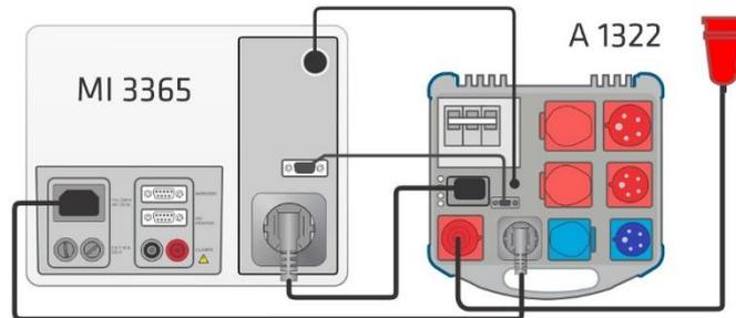
**Figure 9.1: Connecting Active 3 Phase Adapter /plus (A 1322 / A 1422)**
