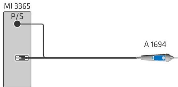
**Figure 9.3: Connecting Tip Commander (A 1694)**
