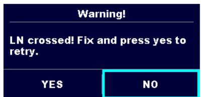
Warning for proper connection in some PRCD measurements. Connection of PRCD's plug must be changed in order to proceed.
