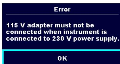
Instrument prohibits the test because 115 V adapter is connected to the instrument and the instrument is powered with 230 V.
