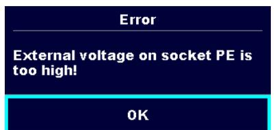
In pre-test a too high external voltage was detected between LN and PE terminals. The measurement was cancelled. Press OK to continue.
