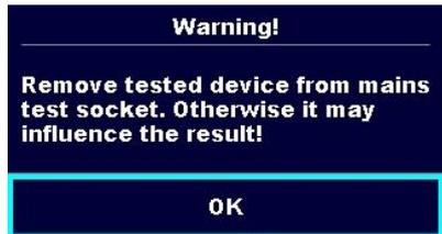
In 2<sup>nd</sup> step of Itou+Ifi test the DUT should be disconnected from mains test socket. Disconnect DUT from mains test socket and press OK to continue.
