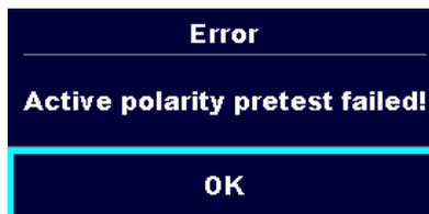
The polarity pre-test of the cable / PRCD has failed. Press OK to continue.
