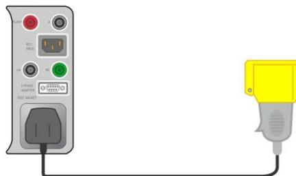
**Figure 9.2: Connecting 110 V Test Adapter (A 1474)**
