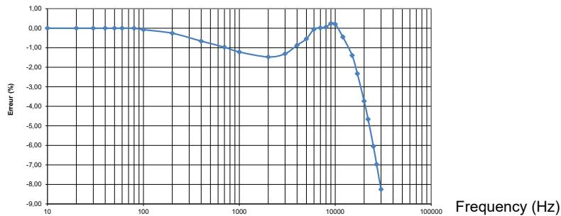
Typical phase versus frequency error curve at 60 A
