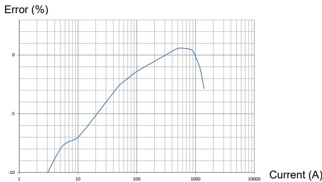
Typical phase error curve at 60 Hz
