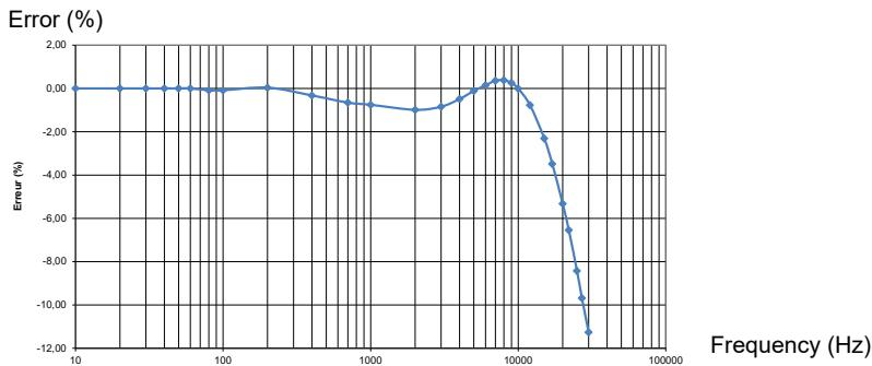
Typical phase error versus frequency curve at 30 A
