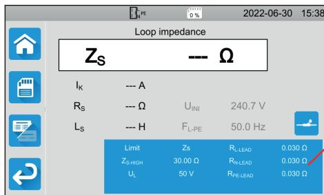
The blue rectangle on the display contains all the settings to configure. They vary according to the measurements.
