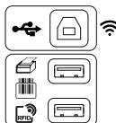
USB type B socket to connect to a PC in order to be able to transfer recorded data or update firmware.
