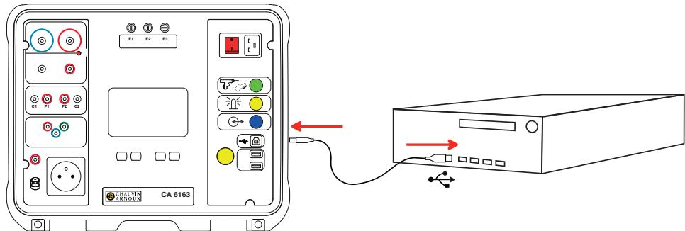
All measurements recorded in the instrument can be transferred to the PC. Transferring data does not erase the saved data.
