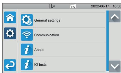
To configure the instrument: select the language, set the date and time and their formats, enable or disable touchpad sound, enable or disable notifications / alarms, adjust display brightness, indicate door checker status for dielectric testing.
